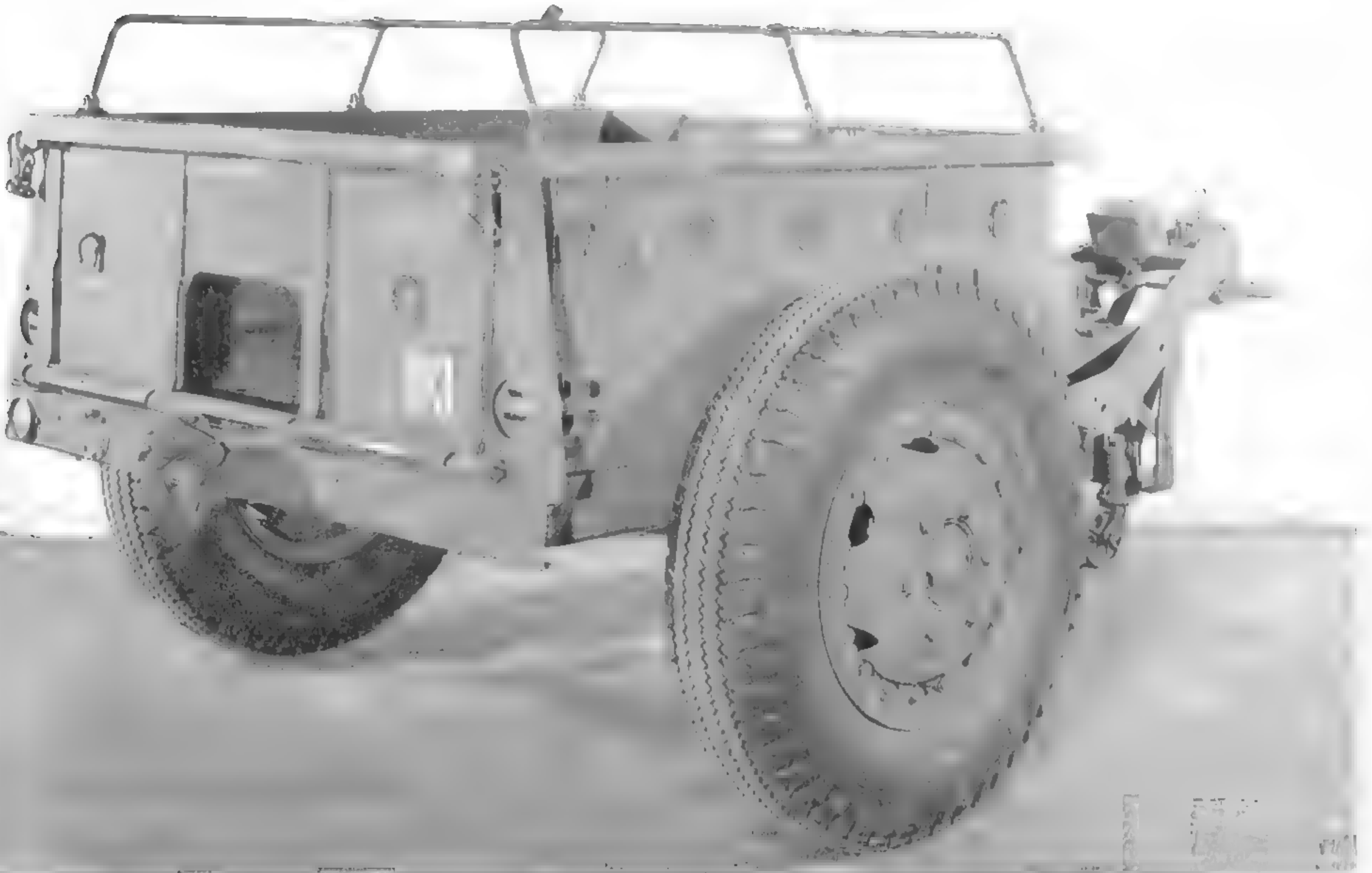
The rear-mounted pintle hook is visible beneath the tailgate, which has a hole cut in it to allow it to be opened fully without interfering with the pintle hook. The bars along the top edge of the trailer sides are intended to support the tarpaulin. (U.S. Army photo)
